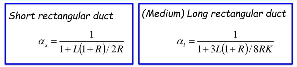
Rectangular duct of any length - empirical equation  $\alpha = \frac{1 + D(L/R)^{E}}{(1/\alpha_{c}) + D(L/R)^{E}} / \alpha_{l}$ where D and E are fitting parameters
